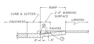
TYPICAL CONCRETE PAVER DETECTABLE WARNING INSTALLATION
